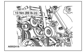
3. Rotate the supercharger belt tensioner clockwise and remove the supercharger belt.
