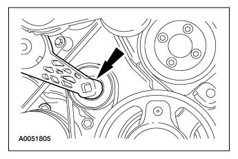
4. Remove the coolant hose assembly bolt.
