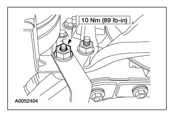
12. Remove the stud and position the coolant hose assembly aside.
