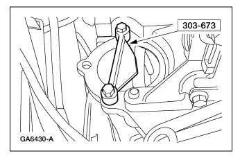
10. Remove the bolts and the alternator support bracket.
