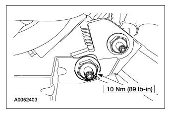
13. Remove the auxiliary crankshaft pulley brace fasteners.
