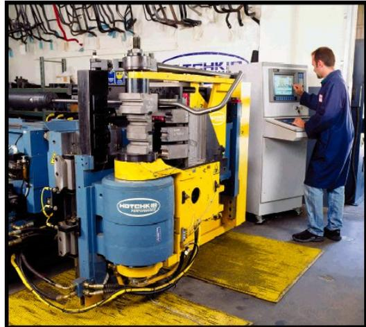
extended production times and higher costs. One final disadvantage is that the press bends can add several extreme tooling dents or 'marks' to the product. Dents such as these are acceptable on a solid bar, but they make the part less eye pleasing to look at. Tubular material *cannot* be bent in this traditional way. The press will either kink or crack the tubing when bending the material.
