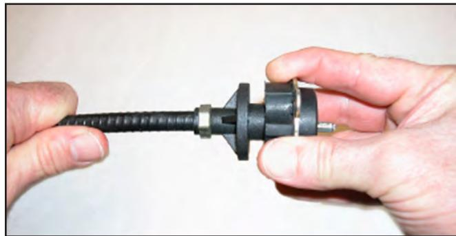
6. Using diagonal cutters, a file or utility knife, remove the four tabs from the end of the housing if present.
