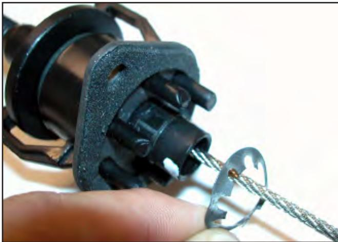
10. Remove the metal/foam gasket from the end of the cable housing.
