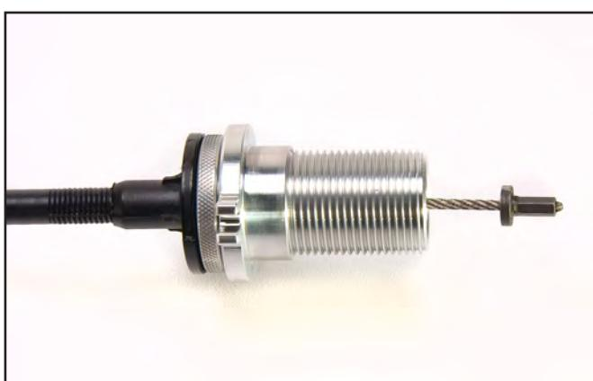
16. Slip the MM Firewall Adjuster over the rubber bushing. Push the firewall adjuster until it is fully seated against the face of the clutch cable housing.
