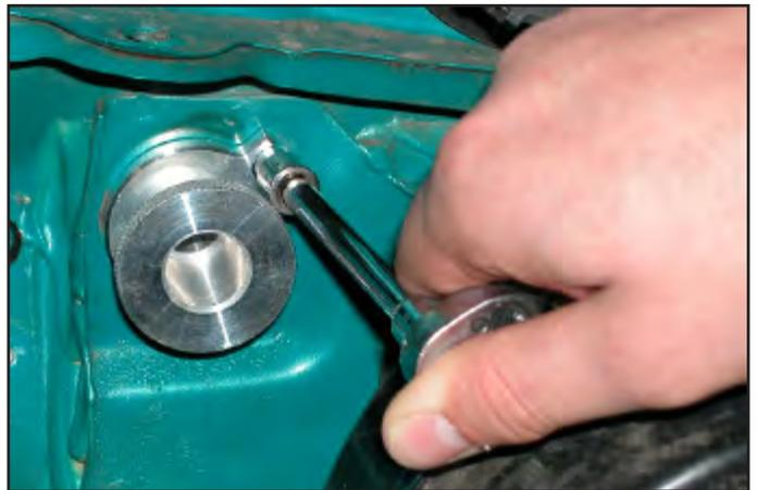
20. Screw the Firewall Adjuster in all the way.
