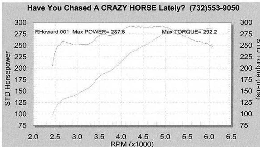
Of course, if 274 horsepower is good, 287.6 is a lot better. And look at that torque curve. We've never seen a [car](#) pick up 15 lbs.-ft. of torque from a cat-back system before.
