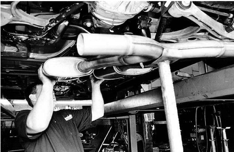
Using a pole jack to support the rear of the setup, O'Malley lined up the dual-mode mufflers to the factory H-pipe.
