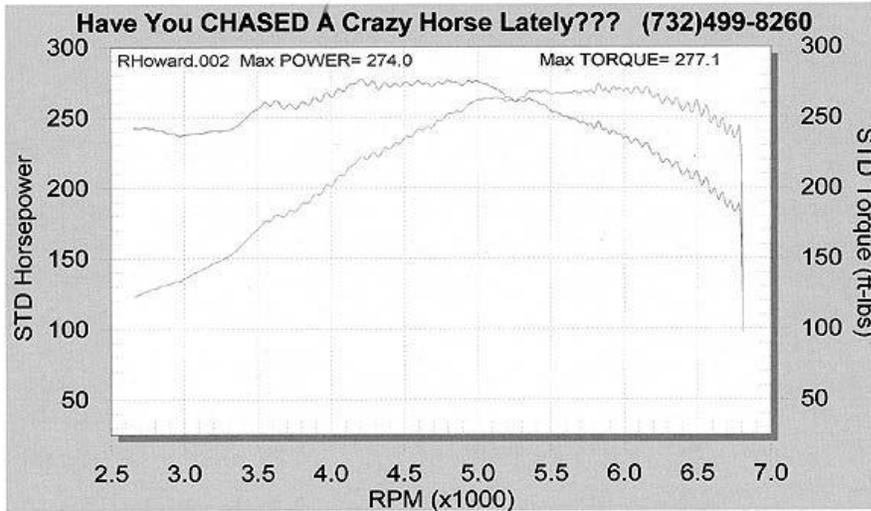
Here's the "before" dyno graph. No doubt, 274 [horsepower](#) from a stock Cobra is nothing to sneeze at, nor is 277 lbs.-ft. of torque. Obviously, the horsepower problems from '99 have been worked out.
