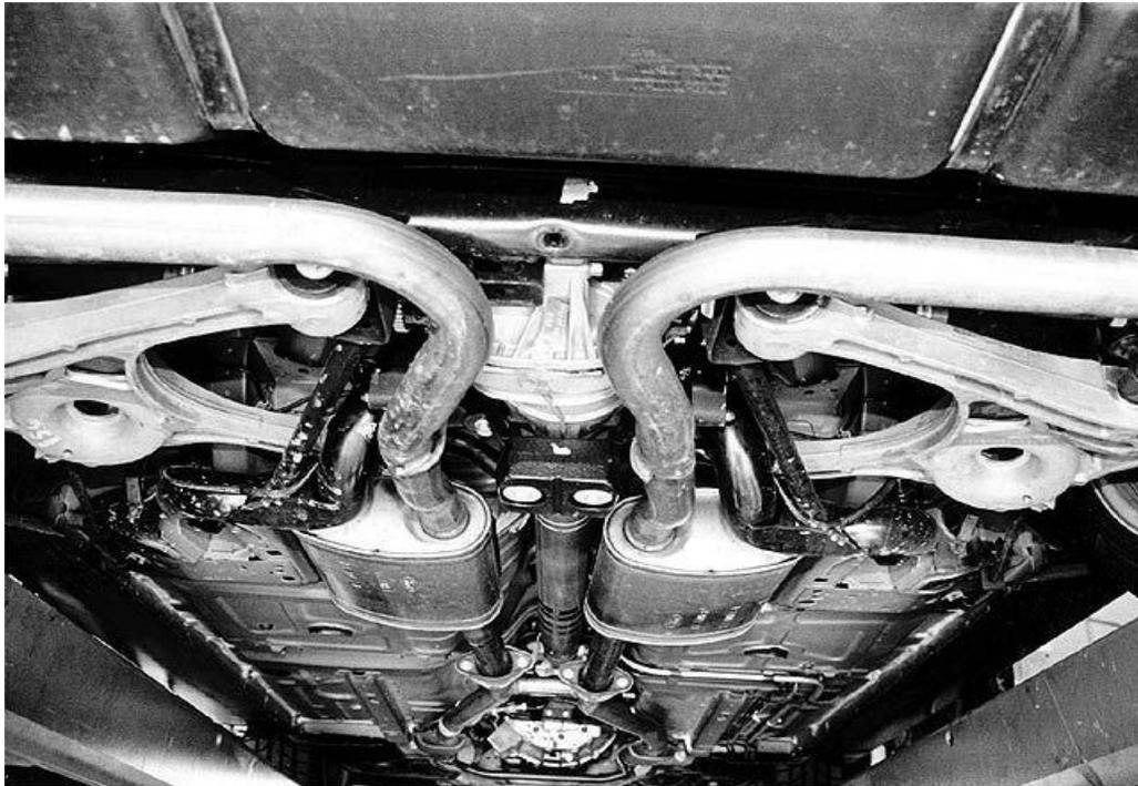
Here's the stock Cobra exhaust system. Note how close the right muffler is to the vibration damper on the differential. The fact that it runs under the IRS made removal a snap.
