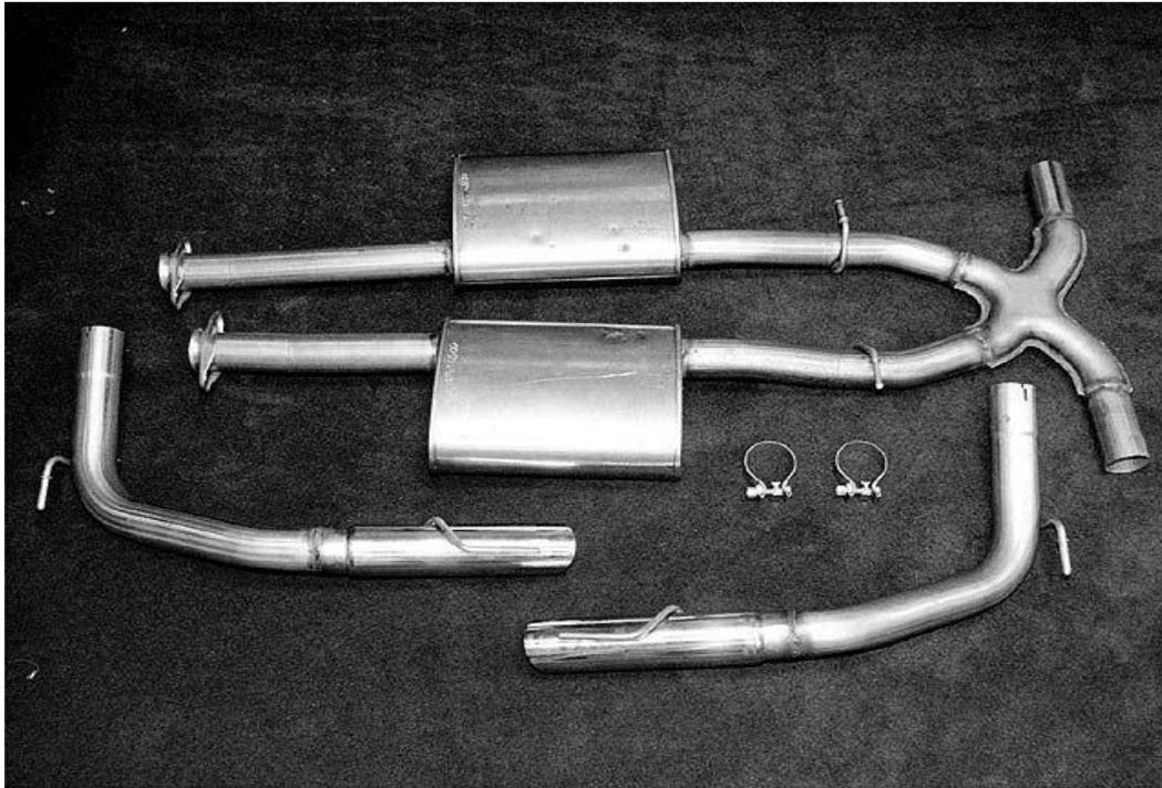
The FR500 kit comes complete with hangers, clamps, bolts, etc. The X-pipe aft of the mufflers cuts down on resonance and adds a bit of [torque](#).
