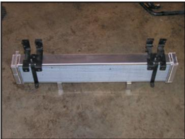
18. Install the AFCO Heat Exchanger asm. into the vehicle just like the factory unit was installed. Install the 4 bolts from the grill opening and tighten.
