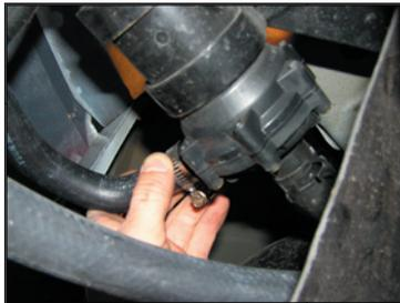
20. Loop the straight 34" piece of hose through the opening in front of the radiator, out below the coolant pump back through the opening in the splash shield and connect one end to the metal line just below the A/C compressor and install the hose clamp.
