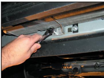
4. Remove the 4 bolts securing the factory heat exchanger to the front mounting brackets.
