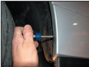
3. Remove the 2 bolts securing the P/S cooler and lower the cooler out of the way.
