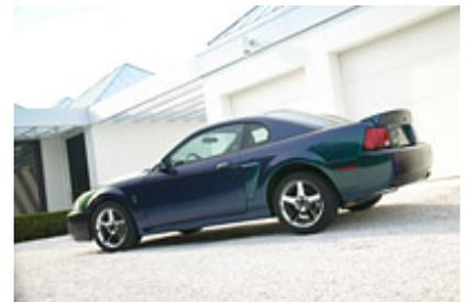
The microscopic layers act like a tiny prism: White light is reflected off the core layer, and then split by outer layers into visible colors. As the viewing angle changes, so does the visible color. The color produced is controlled by precise variances—measured in atoms—in the prismatic layers: The thinnest ChromaFlair pigment shifts from gold through silver and into light blue; The thickest pigment shifts from silver through green, and into purplish blue.
