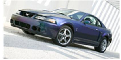
Because ChromaFlair pigments are stirred into a water or solvent base like any paint additive, the paint does not require special handling. As such, Mystichrome paint will be applied at the Dearborn Assembly Plant, using the same process of other factory colors. In addition, Mystichrome passes the same rigorous durability tests of any factory paint. Also, the dramatic color shifts actually hide paint applied during body repair.
