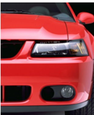
New front face fascia helps deliver more air to the engine for intake and cooling systems.
