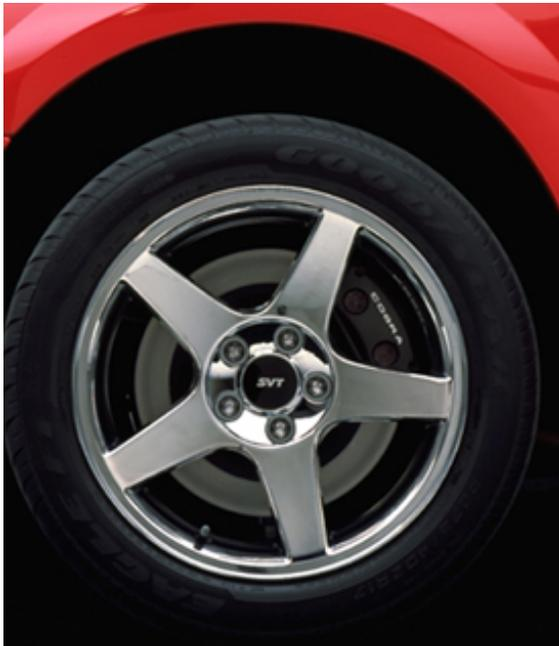
New cast-aluminum 17 x 9-inch wheels are fitted with 275/40ZR-17 Goodyear Eagle F1 tires. The braking system includes 13-inch Brembo™ front rotors with PBR™ dual-piston calipers, and 11.65-inch rear rotors with single-piston calipers. The pad material on the rear brakes has been upgraded for enhanced durability and brake performance.
